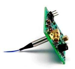
This optical detector amplifier is designed as a generic daughterboard for integration into custom systems. It can be used as an optical power meter or mounted on a custom PCB as part of the system. The amplifier's gain can be varied by a turning pot in 10dB steps. Customers can select a cost-effective detector for performance verification.
